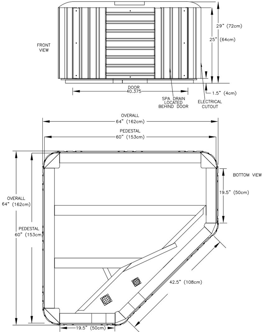
**NOTE:** Watkins Manufacturing Corporation recommends that the Aventine be installed on a minimum 4" thick reinforced concrete pad or structurally sound deck able to support the "dead weight" found in the spa specification chart.
