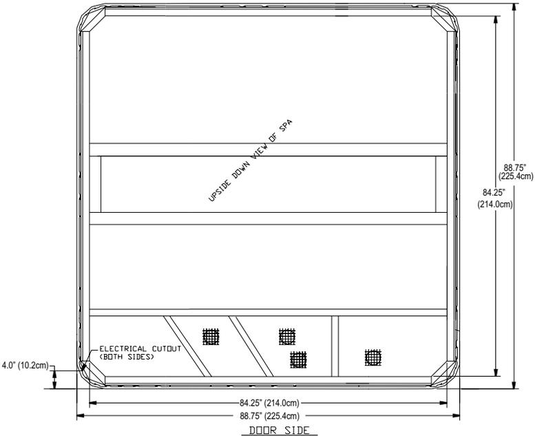
**NOTE:** Watkins Manufacturing Corporation recommends that the Palatino be installed on a minimum 4" thick reinforced concrete pad or structurally sound deck able to support the "dead weight" found in the spa specification chart.
