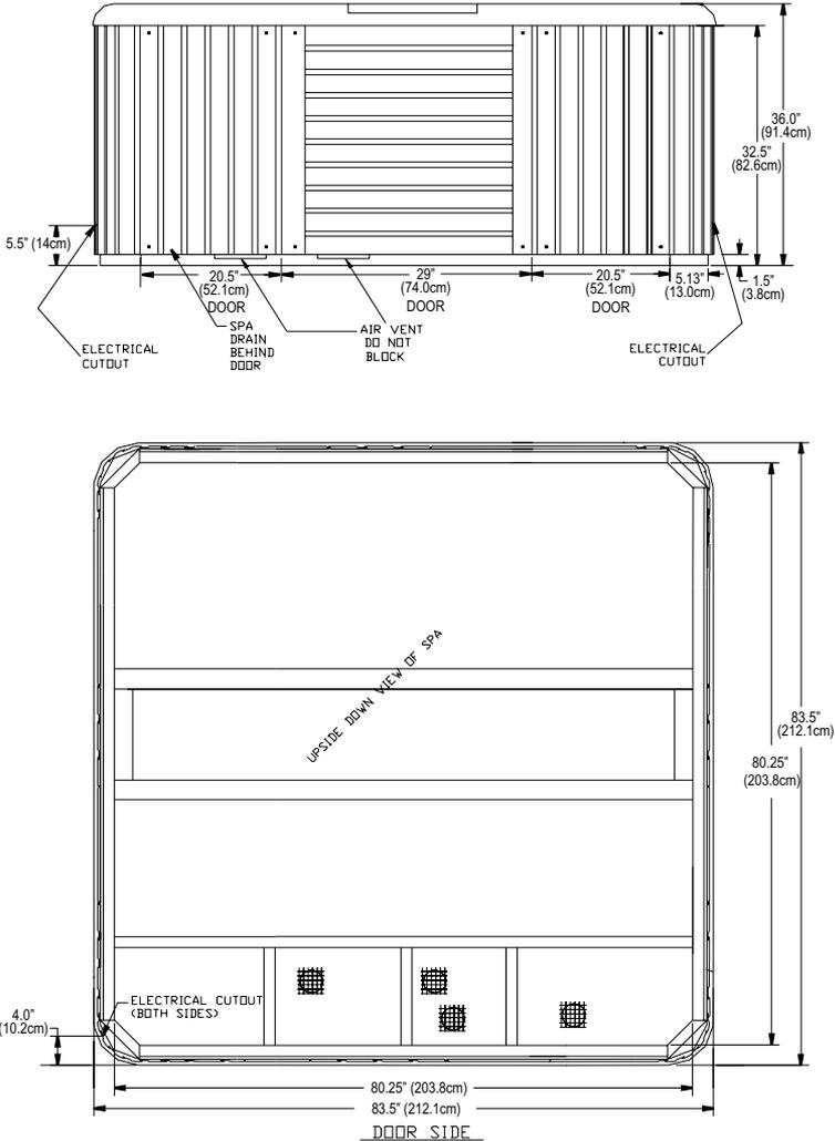
**NOTE:** Watkins Manufacturing Corporation recommends that the Marino be installed on a minimum 4" thick reinforced concrete pad or structurally sound deck able to support the "dead weight" found in the spa specification chart.
